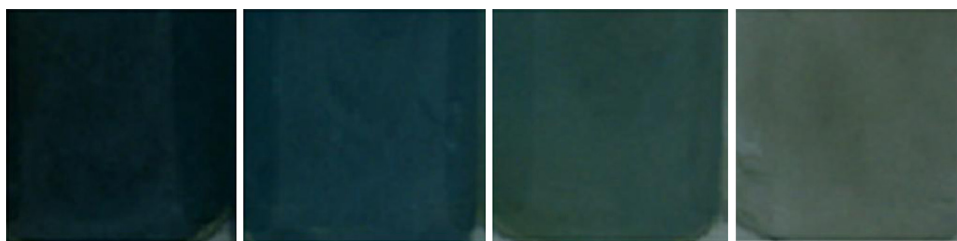
Fig. 4. Photographic images of fibres A0.30, A0.35, A0.40, and C, left-to-right, after staining with 0.01% (w/v) Amido Black 10B aqueous solution for 12 h.
